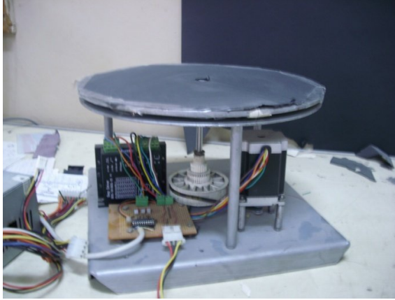
Figure 1. The rotary table is used in our work to change the camera's viewing direction to an object.
