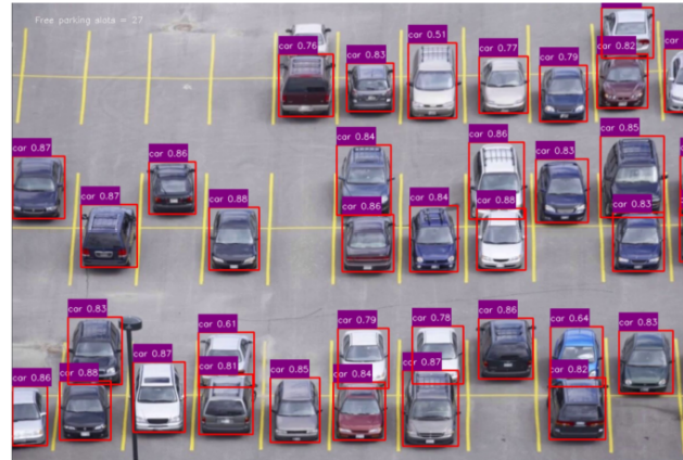
Figure 16. Detection result in a 66-space parking area using YOLO V8s
