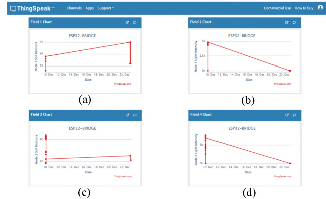
Figure 19. Data Display on Thingspeak (a) Node 1 Soil Moisture (b) Node 1 Light Intensity (c) Node 2 Soil Moisture (d) Node 2 Light Intensity
