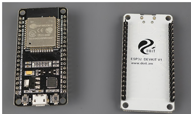
Figure 3. ESP32 DEVKIT V1 module board [20]
