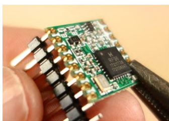
Figure 4. LoRa Hope-RFM9x wireless communication [27]
