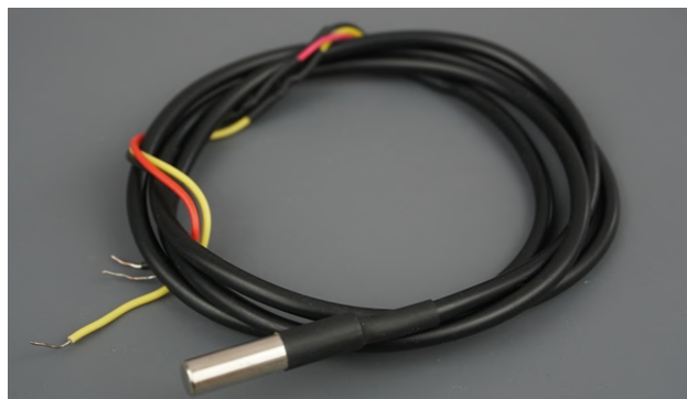
Figure 6. DS18B20 digital temperature sensor [28]
