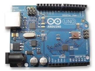
Figure 3. Arduino Uno microcontroller
