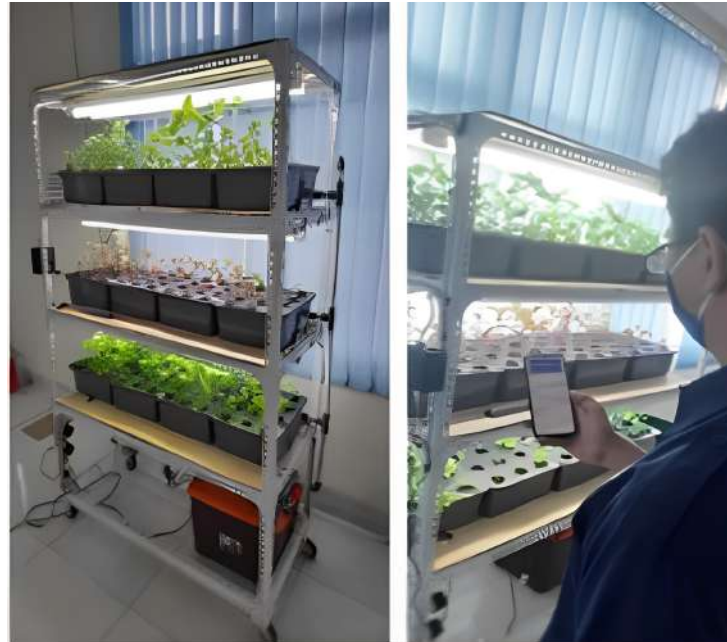
Figure 5. IoT-enabled Indoor Hydroponics System
