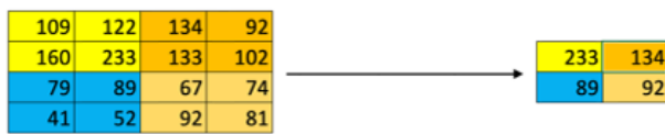
Figure 3. Pooling layer process to calculate new feature map based on maximum value of specific area in feature map
