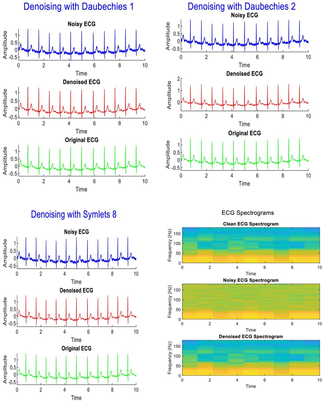
Figure 7. Displays the denoising performance of different mother wavelet functions (MWF) for ECG signals. Symlets and Coiflets MWFs outperform Daubechies MWF in terms of noise reduction, with spectrogram analysis confirming the elimination of high-frequency noise components.
