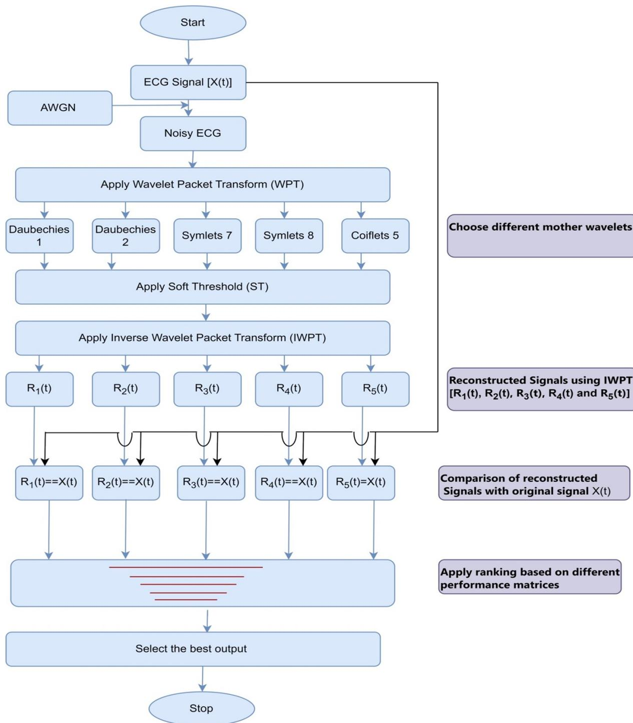
Figure 6. Flowchart depicting the proposed technique for eradicating AWGN from ECG signals.
