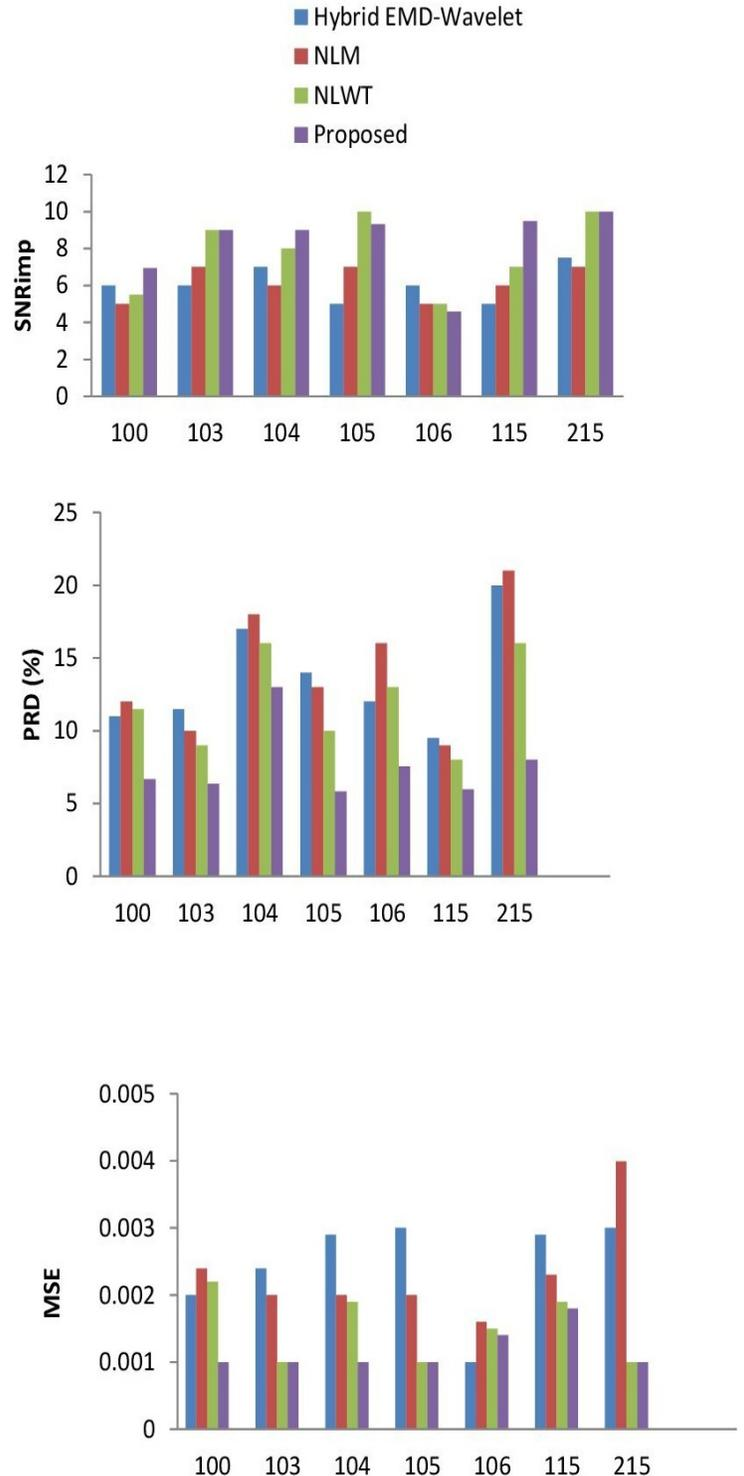
Figure 9. Denoising Performance Proposed Algorithm on different Records from MIT-BIH Database at 20 dB SNR
