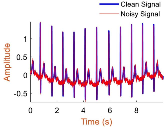
Figure 5. Comparison of the original noisy ECG signal with the processed denoised ECG signal acquired by employing the proposed Wavelet Packet Transform-based denoising approach.
