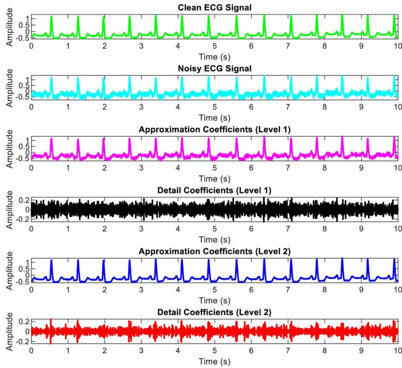
Figure 10. Steps involved in Denoising of Proposed Algorithm on Record 105 from MIT-BIH Database
