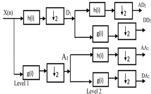
Figure 3. Two level decomposition, using WPT
