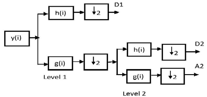
Figure 1. Signal analysis two-level 1D DWT Decomposition filter model
