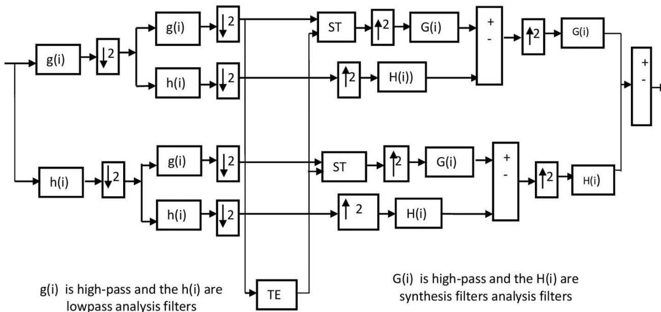
Figure 4. Real-time WPT architecture block diagram for signal denoising
