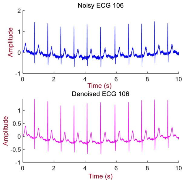
Figure 8. Denoising Performance of Proposed Algorithm on Record 106 from MIT-BIH Database at 20 dB Input SNR
