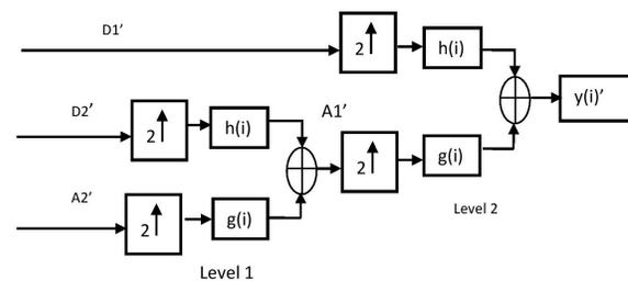
Figure 2. Signal synthesis two-level 1D IDWT Decomposition filter model
