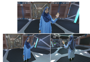
Figure 7. Results of the proposed 3D reconstruction method in MR telepresence; (a) front view; (b) side view; (c) back view
