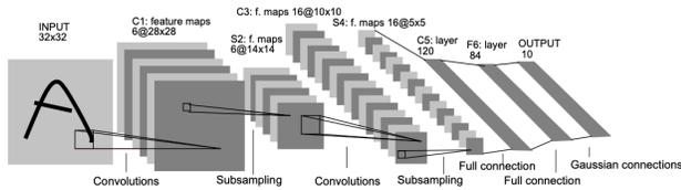
Figure 1. The first CNN architecture, LeNet from [22]
