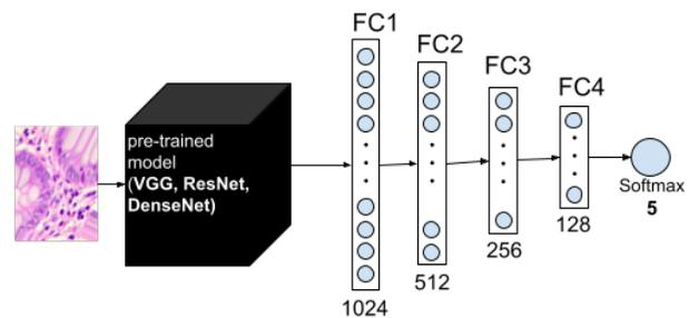
Figure 2. the structure of model (3) using a pre-trained model and four fully connected layers.
