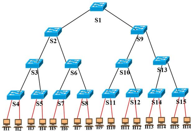
Figure 7. Tree Topology (Depth 4, Fanout 2).
